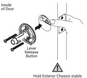
while installing Interior Chassis
