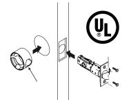
Lockset 1. Place the steel cup inside the 2/18" hole in the door as shown. The open part of the cup is now to qulify as an UL approved lockset the steel cup must be installed as part of the unit.
