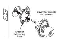
Align rose support in door in a vertical position. Insert square spindle through square hole in latch and install chassis over the latch.
